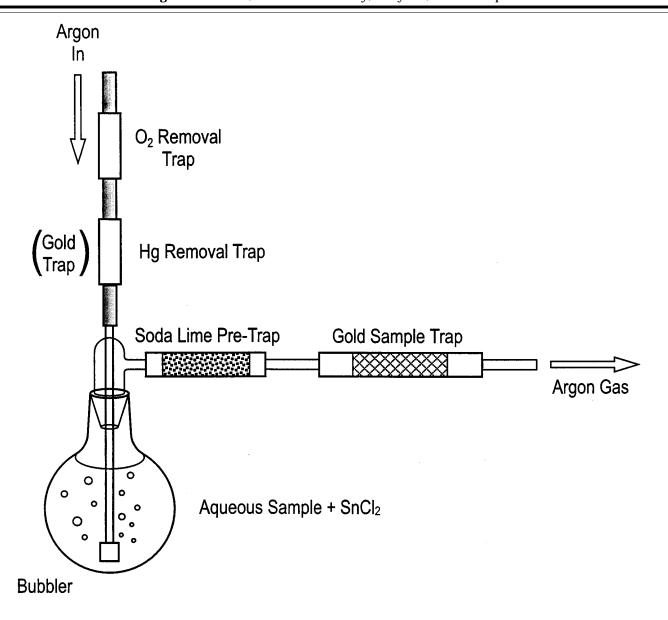
Figure 1. Schematic Diagram of Bubbler Setup
