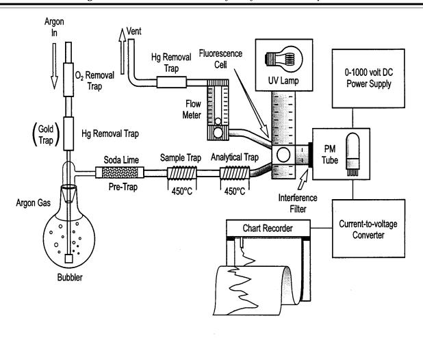
Figure 2. Schematic Diagram of the Cold Vapor Atomic Fluorescence Spectrometer (CVAFS) System
